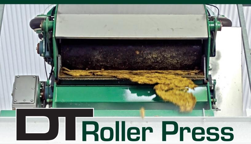
The DT Roller Press is manufactured with heavy duty construction for longevity and strength against the most demanding applications. The press rolls are designed with advanced rubber roller vulcanization and are each individually driven to prevent slippage and stalling from large objects. Our DT Roller Press also has reinforced backing on the screen roller for added strength as well as a remote grease bank.
