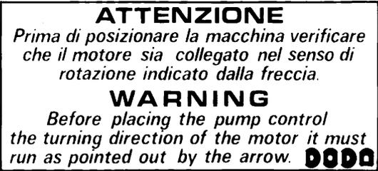
THIS STICKER REMINDS YOU TO CHECK THE ROTATION SENSE OF THE MACHINE ELECTRIC MOTOR BEFORE STARTING THE MACHINE.
